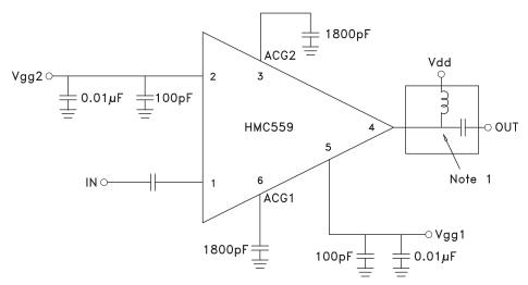
NOTE 1: Drain Bias (Vdd) must be applied through a broadband bias tee with low series resistance and capable of providing 500mA
